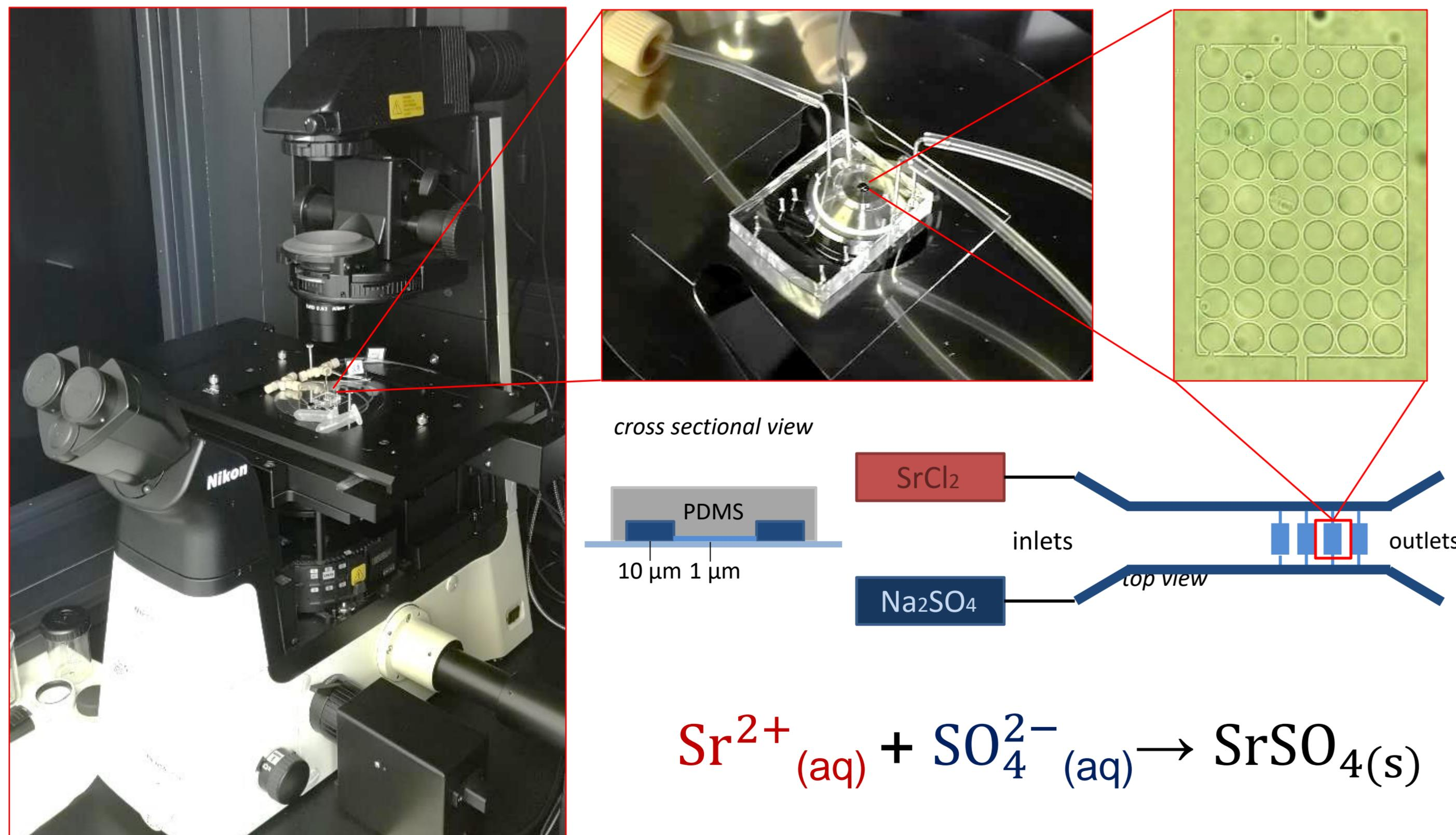
Microfluidic chamber to precipitate celestine ( $\text{SrSO}_4$ ) from the mixing of  $\text{SrCl}_2$  and  $\text{Na}_2\text{SO}_4$  solutions
