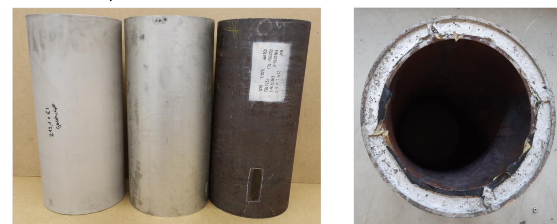
Pre-Test are performed on exposed and concreted- in pipes
