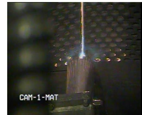
Up to 200mm in thickness in air (14kW laser power)
