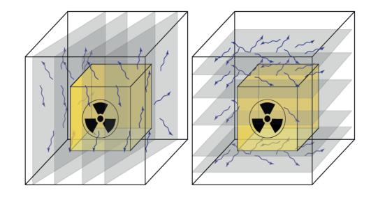
Fig. 2: Potential fluid pathways within granitic host rocks resulting from extensional fracturing are highly dependent on the anisotropic fabric of the granitic material. It is determined by various geological processes such as magmatic flow, static crystallisation, plastic deformation, post-intrusive hydrothermal processes, etc.
