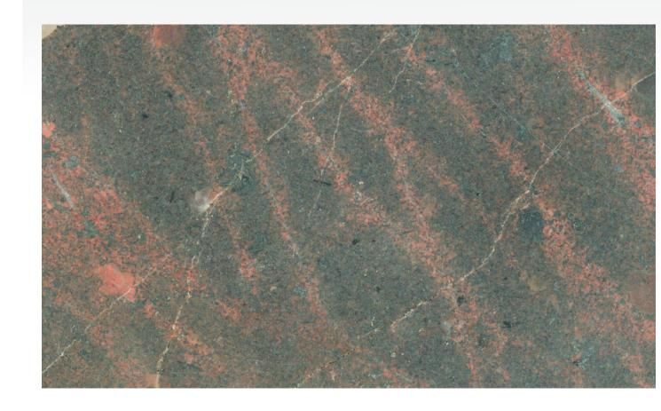
Fig. 8 (left): Niederbobritzsch granite, fractures with alteration zones (annealed) and open, younger fractures.
