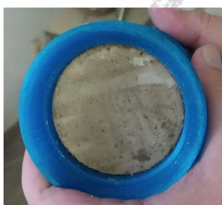
Compacted clay in the cell
