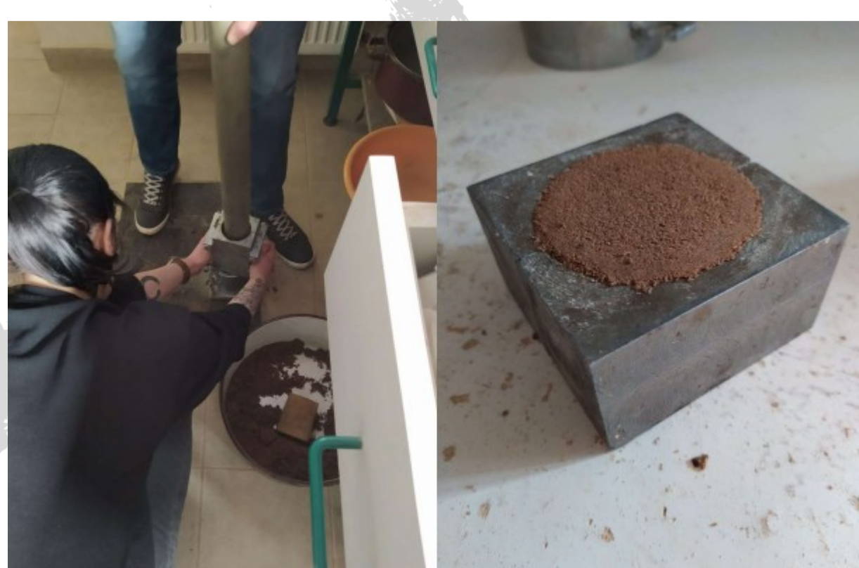
Sample compaction (Proctor test) and compacted mixture of sodium bentonite and quartz sand in mold
