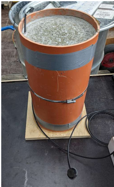
One SensorNode (blue) has been embedded at the bottom of a 40cm-height pipe and one (orange) is outside to monitor the external environment.
