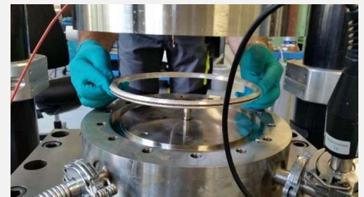
Figure 6: Lifting/repositioning of the seal before repeated compression
